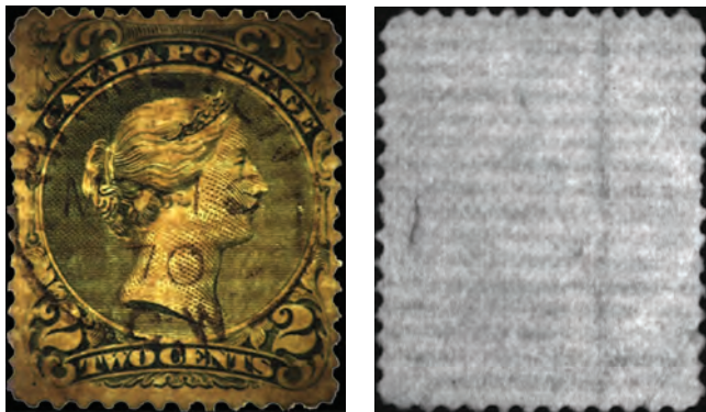
FIGURE 3. Laid lines using the VSC 6000 as seen from front with 365nm transmitted ultraviolet light, and from the back using spot fluorescence.
