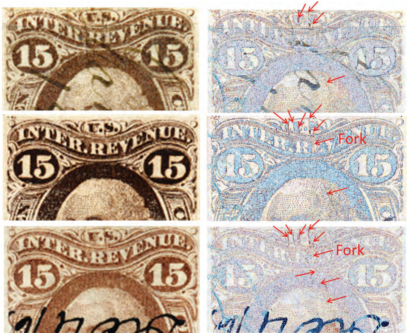
FIGURE 3. An example using subtraction to highlight poorly visible plate-crack detail on the First Issue 15 cent Inland Revenue Documentary stamp. Since the features to be enhanced are faint, 24-bit color images are used instead of thresholded, false color images with gray scale. Views of the multiple cracks and a fork in the crack are significantly enhanced by the subtraction. The crack traversing the hair in the portrait is visible on all three stamps after subtraction.
