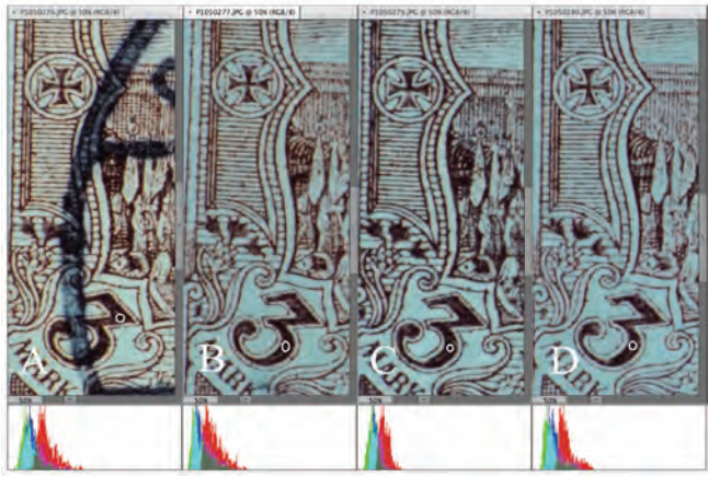
FIGURE 9. 34b: Michel Offices in Turkey number 34 stamps exhibiting red orange in UV tonal histograms from “water drop” selections (white circles indicate approximate sites) of the left postal values. Numbers of selected pixels ranged from around 350 to 750 for all samples. B: item sold as 34a. C: item signed 34b.
