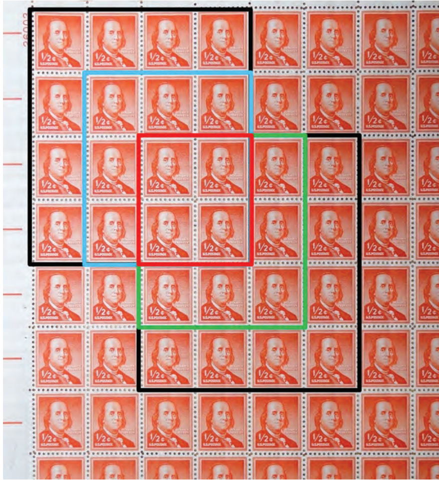
FIGURE 9. Overlapping blocks for comparing the calculations of the relative distortion patterns using different numbers and choices of stamps.
