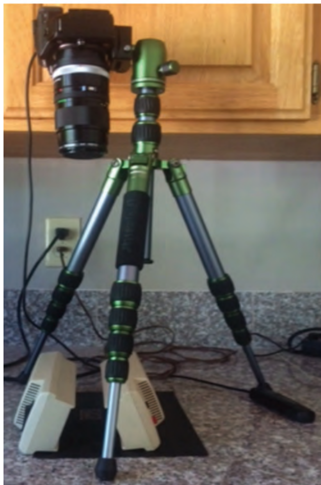
FIGURE 3. Set-up for UV photographs. The camera is mounted on a tripod and focused on a stamp located on a black background between two 40-watt UV (365 nm) lamps. Exposure is made with a remote shutter seen lying against the right-most leg of the tripod.
