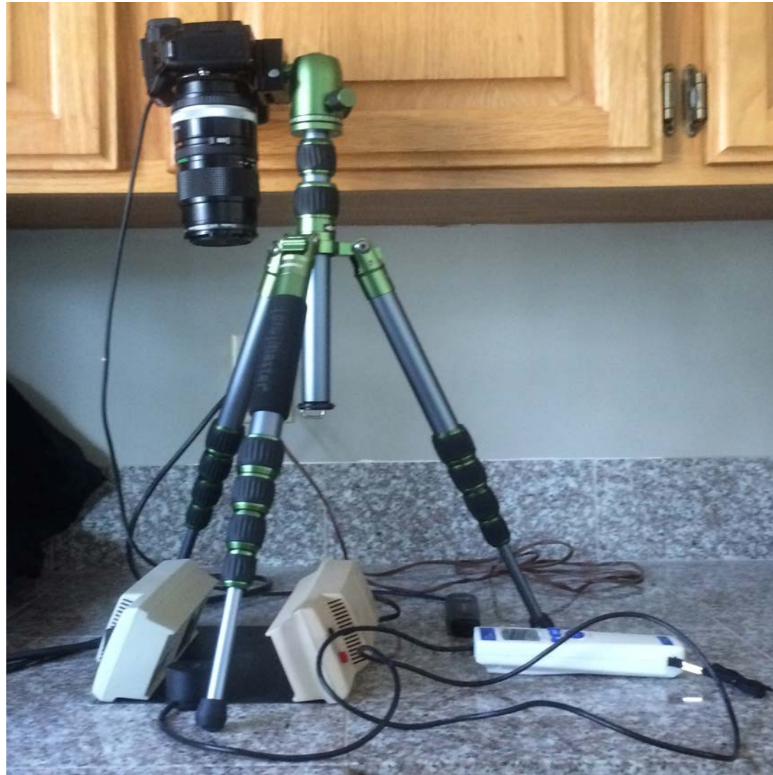
Camera and attachments for making UV photographs.
