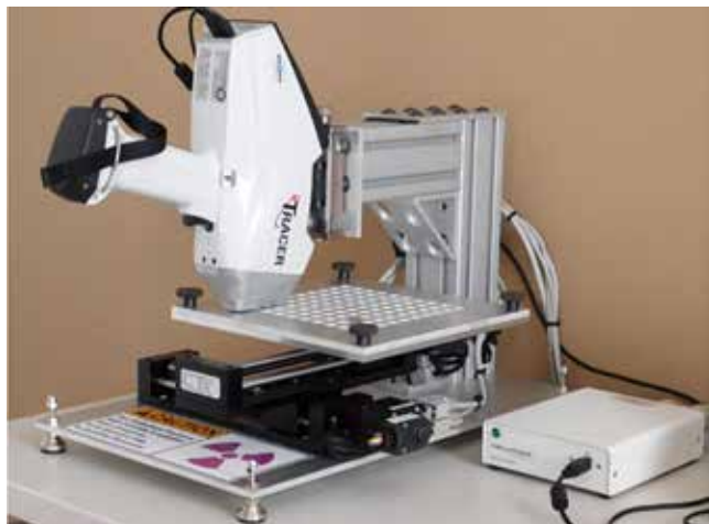
Figure 1. DeWitt MSS-150E scanning stage with the Bruker Tracer 5i attached.
