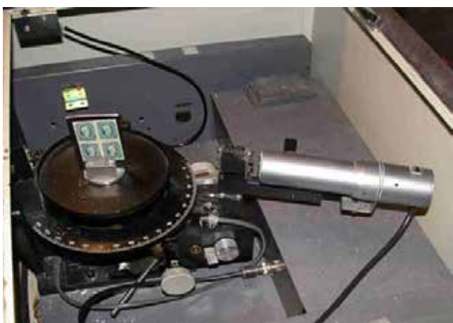
Figure 1. Interior view of the X-ray diffractometer, illustrating the goniometer and the mounting relationship of a studied stamp with the X-ray source (extreme left of the figure) and the detector (the cylindrical object at the right side of the figure).
