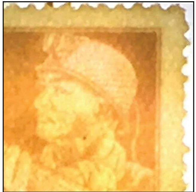
FIGURE 4. Stamp photographed by transmitted light shows pattern from the wire web characteristic of machine-made paper.
