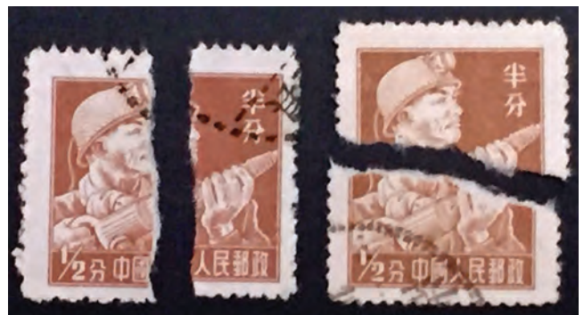
FIGURE 3. Stamps torn vertically and horizontally show characteristic patterns for machine-made paper.
