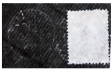
Portion of a cover and stamp, normal and beta ray image showing watermark
