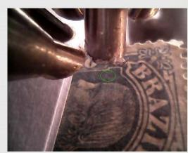
The main difference between XRF and PIXE analyses is the depth of the rays in the sample.
