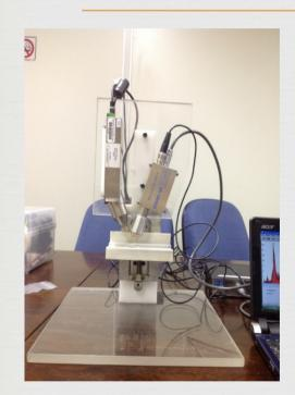
The X-Ray Fluorescence Analyzer – XRF – is a non-destructive analysis technique, which has been widely used to investigate the elemental composition present in certain materials, including in postage stamps.
